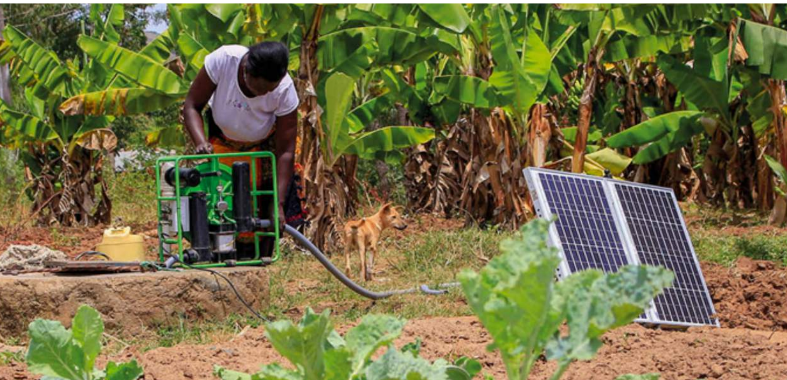
Farmer using a solar irrigation pump equipped with a sensor. ©Futurepump
